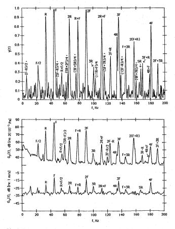
Fig. 2 Coherence  $[\gamma(f)]$ , radiated noise spectrum  $[G_p(f)]$ , and fluctuating velocity spectrum  $[G_v(f)]$  with horizontal anemometer sensor.
