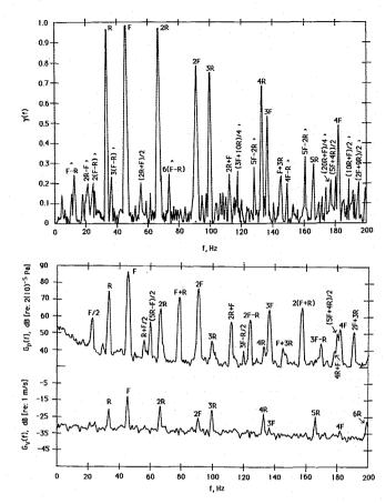
Fig. 1 Coherence  $[\gamma(f)]$ , radiated noise spectrum  $[G_p(f)]$ , and fluctuating velocity spectrum  $[G_v(f)]$  with vertical anemometer sensor.
